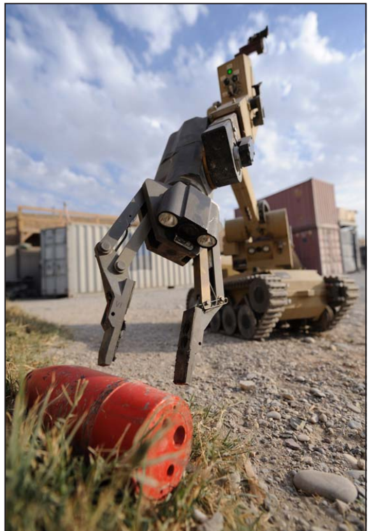
The Explosive Ordnance Detection robot, "tEODor", employed by the Kandahar Provincial Reconstruction Team, is a remote-controlled manipulator vehicle used for locating, inspecting and investigating unknown objects and also for the deactivation and destruction of any explosive devices that are found. (Canadian Forces photo by Master Corporal Angela Abbey)
